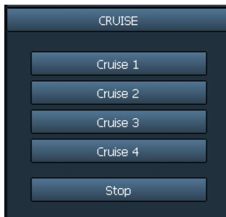
Click "cruise" button, it displays cruise control panel. Different PTZ calls different preset cruise. For example: PTZ call preset 101 to start cruise group 1. You can save the corresponding preset position of **【cruise 1】** button. If need to start the cruise, click **【cruise 1】** . Cruise button setting as below:
